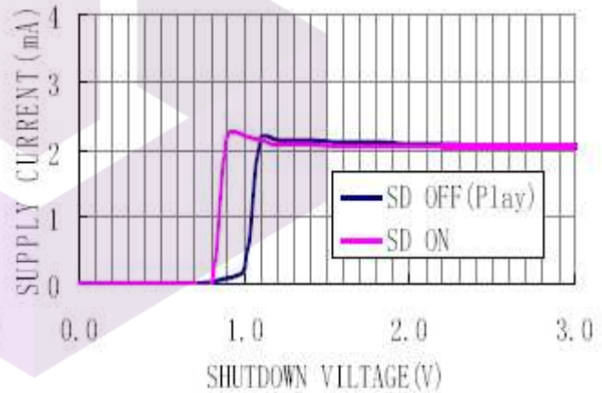
Shutdown Hysteresis Voltage VDD=3.3V
